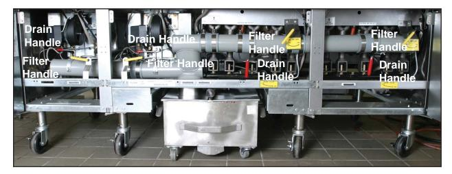
Above is an annotated view of the handles for the filter and drain operation unique to this unit. A quick reference for filtration of the unit is provided to the right and below.
